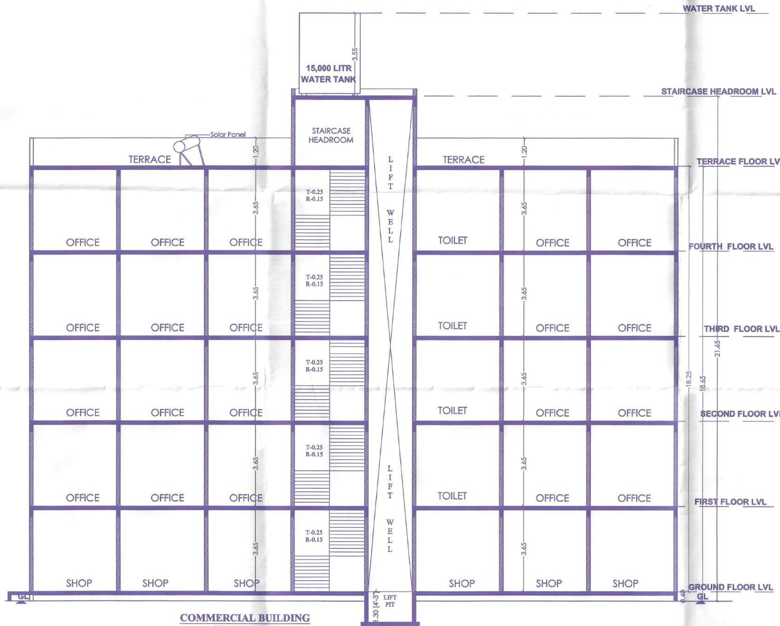
COMMERCIAL BUILDING SECTION-EE
