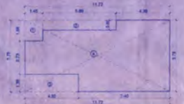
BUILT UP AREA LINE DIAGRAM FOR SAMPLE FLAT SCALE: 1:100
